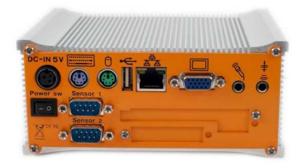
On the back of the appliance you can connect a monitor using a standard VGA cable, a PS2 keyboard and a mouse. If you don't have a PS2 keyboard then you can also use an USB keyboard using the USB port on the front. When connected you will be prompted with a standard windows login screen as shown below.
