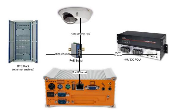
As shown in the above picture, a RJ45 cable is connected from the appliance to the switch. Same goes for the PDU and camera. For the camera make sure to plug it into of the switche's PoE ports.
