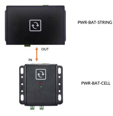
3.4. For connecting more than one PWR-BAT-CELL, just connect the OUT port of the first PWR-BAT-CELL to the IN port of the next PWR-BAT-CELL, repeat this process until the last PWR-BAT-CELL.
