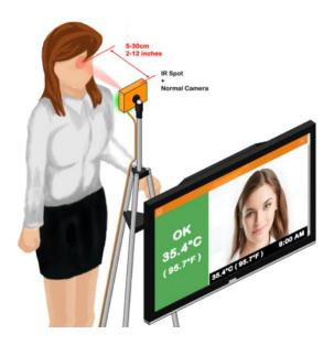
• **EST-IRSPOT-THERMAL** - With the optional thermal camera, the entire face will be scanning in 480 points instead of just one measurement with the IR spot sensor. The hottest detected temperature will be retained. This ensures that the entire face is screened.
