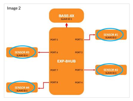
For instance, if Sensor #1 is connected to port 1 and Sensor #2 is connected to port 3, the Slave ID #2 will be assigned to the first sensor connected, in this case, Sensor #1. This dynamic assignment ensures efficient communication and management of multiple sensors within the system. The same rule applies for sensors connected directly to the Base Unit.
