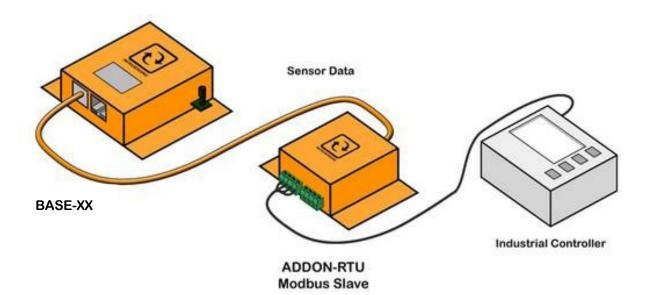
Below is an image of the wiring diagram for us to connect our control
