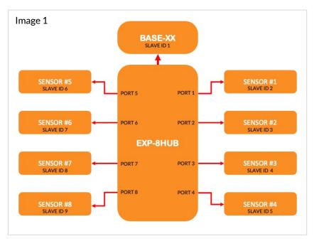
For example, let's consider a scenario where there are four sensors connected to the expansion hub, each connected to different ports. In this case, the Slave ID number will be assigned according to the port to which each sensor is connected.
