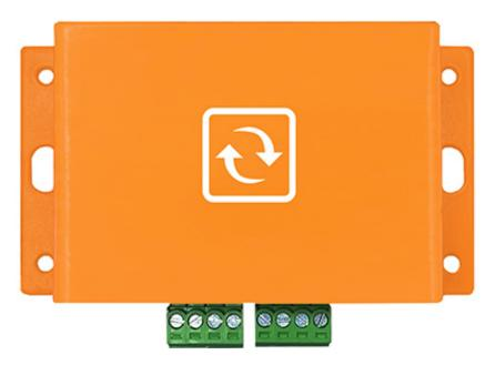
The Add-On connects like a typical sensor to any of the external sensor ports of our Base Unit (BASE-XX) or our Expansion hubs (EXP-8HUB/EXP-4HUB) and then your controller is connected to the RTU Add-On via RS-485
