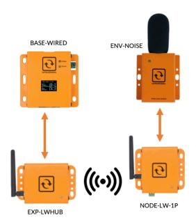
You can wirelessly connect your sensor probe to the BASE-WIRED, each LoRa hub can support up to 20 LoRa node. The LoRa Hub's power is supplied by the BASE-WIRED while the LoRa Node's power can be supplied by 12/24V DC or a USB-C type.
