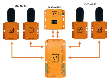
You can connect up to 8 sensor probes to the BASE-WIRED using the EXP-8HUB
